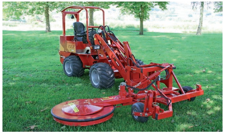
Large swing reach, Hyd. height adjustment, spring tensioner
