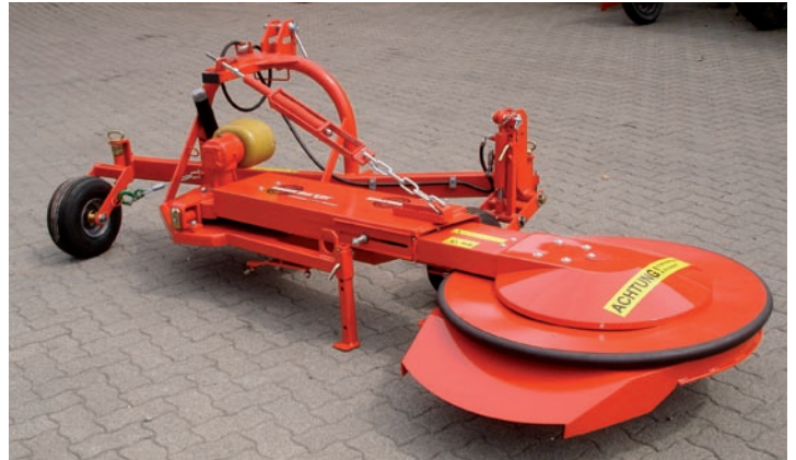
Low mowing head enables mowing under low fences
