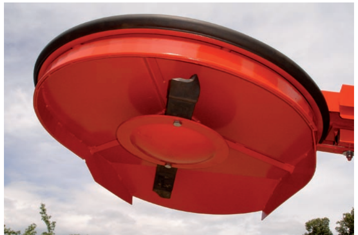
Slide plate under the knives minimizes damage to the grass roots
