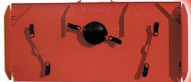
Swinging blades and skid plate under the middle rotor are standard
